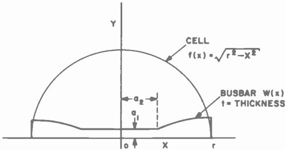
Fig. 4—Coordinate axis and geometry for a double ended bus bar, current extracted at both ends. The  $y$ -axis scale for  $W(x)$  has been expanded for clarity.
