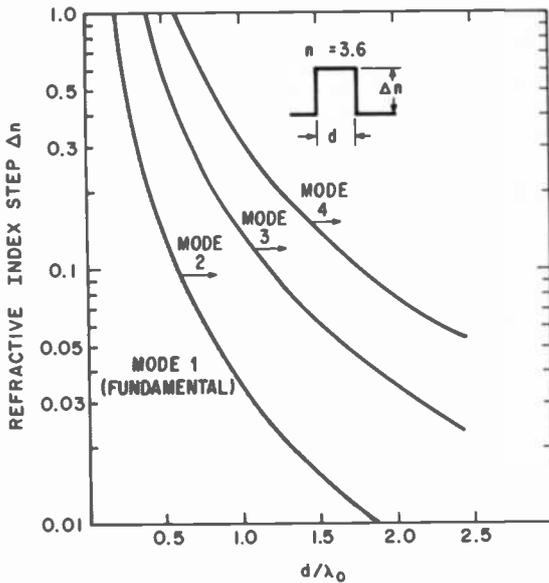
Fig. 4—Modal cutoff conditions for symmetric double-heterojunction lasers. The fundamental mode can propagate for all value of  $\Delta n$  and  $d/\lambda_0$ , but for waveguides defined by points lying to the right of each curve, high order mode propagation is possible.
