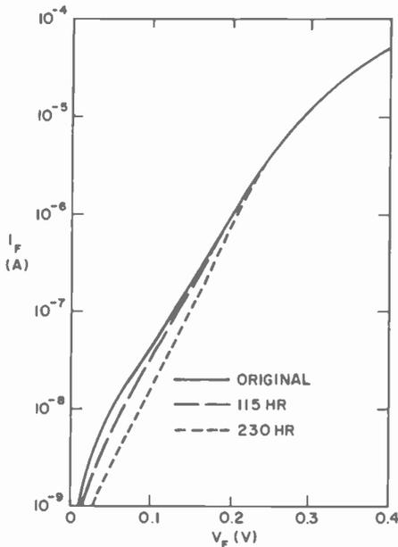
Fig. 5—Forward  $I$ - $V$  characteristics of a Schottky diode showing the excess current reduced by BT tests.
