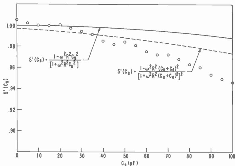
Fig. 7—Relative incremental sensitivity  $S'(C_S)$  versus  $C_S$ .
