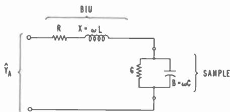
Fig. 4—Simplified equivalent circuit of sample and BIU.
