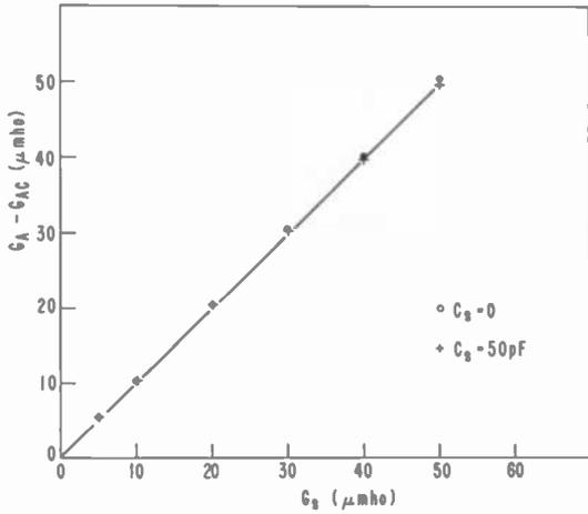
Fig. 9—Conductance  $G_A - G_{AC}$  versus standard conductance  $G_S$  for  $C_S = 0$  and 50 pF.
