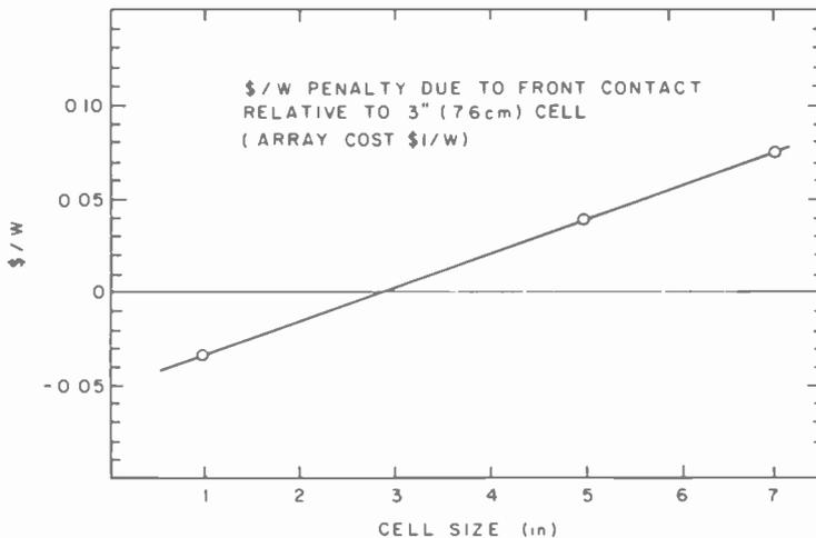
Fig. 3—Calculated penalty in  $\$/W$  due to combined cost and performance contributions of optimum fine grid and bus bar on cell front as a function of cell size. The penalty is shown as a change from a reference array cost of  $1\$/W$  for all cell sizes with the zero arbitrarily set at the 3-inch (7.6 cm) wafer.
