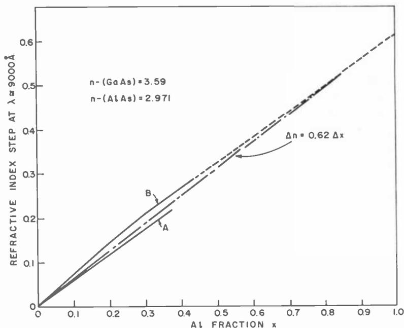
Fig. 1—Refractive index step (at 9000 Å) at an  $\text{Al}_x\text{Ga}_{1-x}\text{As}/\text{GaAs}$  heterojunction as a function of  $x$ . Curve A is from Ref. [4] and curve B is from Ref. [3].
