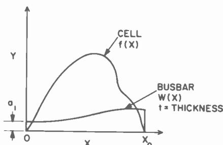
Fig. 1—Coordinate axes and geometry of the problem. The  $y$ -axis scale for  $W(x)$  has been expanded for clarity.
