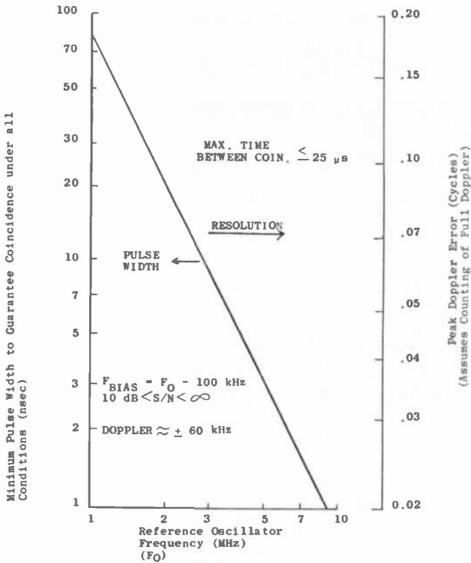
Fig. 12—Minimum pulse width to guarantee coincidence for all conditions.
