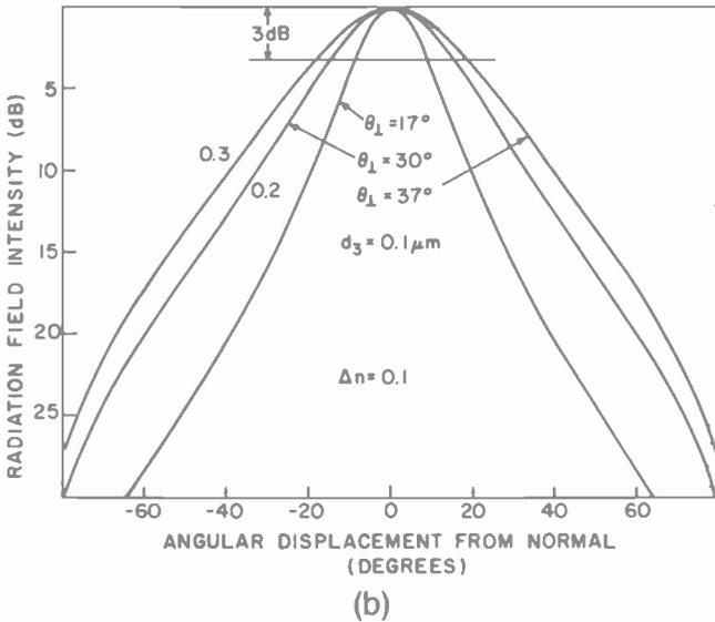
Fig. 7—(a) Field intensity as a function of waveguide width  $d$  for  $\Delta n = 0.1$ ; (b) corresponding far-field. Here  $\lambda_0 = 0.9 \mu\text{m}$ .
