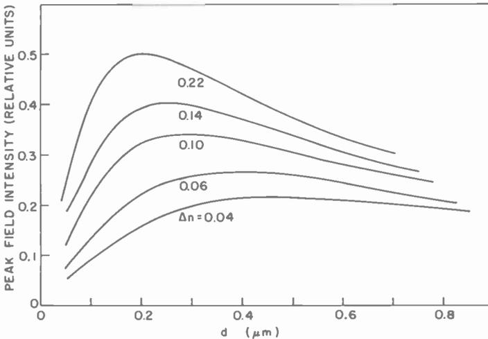
Fig. 9—Peak field intensity as a function of  $d$  for several values of  $\Delta n$ . Here  $\lambda_0 = 0.9 \mu\text{m}$ .
