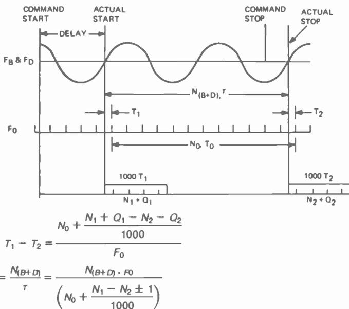
Fig. 10—Analog technique for reduced quantization error.
