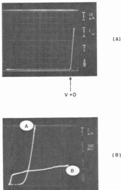
Fig. 1—The current-voltage characteristics of a typical Al-SOS Schottky diode.
