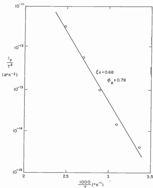
Fig. 3— $\log I_F$  versus  $1/T$  plot of an Al-SOS Schottky diode.
