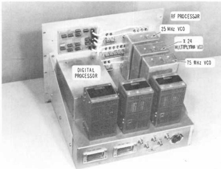
Fig. 13—One-way Doppler extractor chassis.
