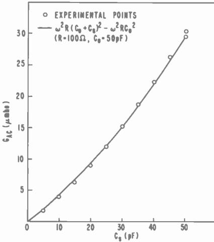
Fig. 8—Apparent conductance  $G_{AC}$  versus  $C_S$ .
