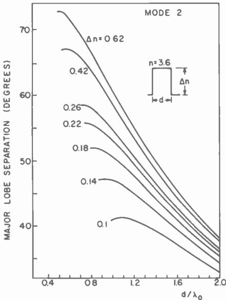
Fig. 5—Major lobe separation in the far-field for device operating in the second mode as a function of the index step  $\Delta n$  and  $d/\lambda_0$  (symmetric structure).
