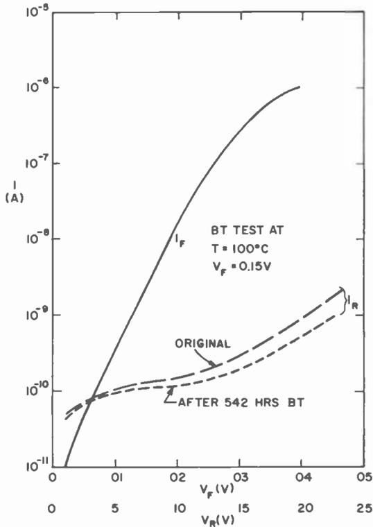
Fig. 6— $I$ - $V$  characteristics of a Schottky diode before and after BT tests with  $V_F = 0.15$  V.
