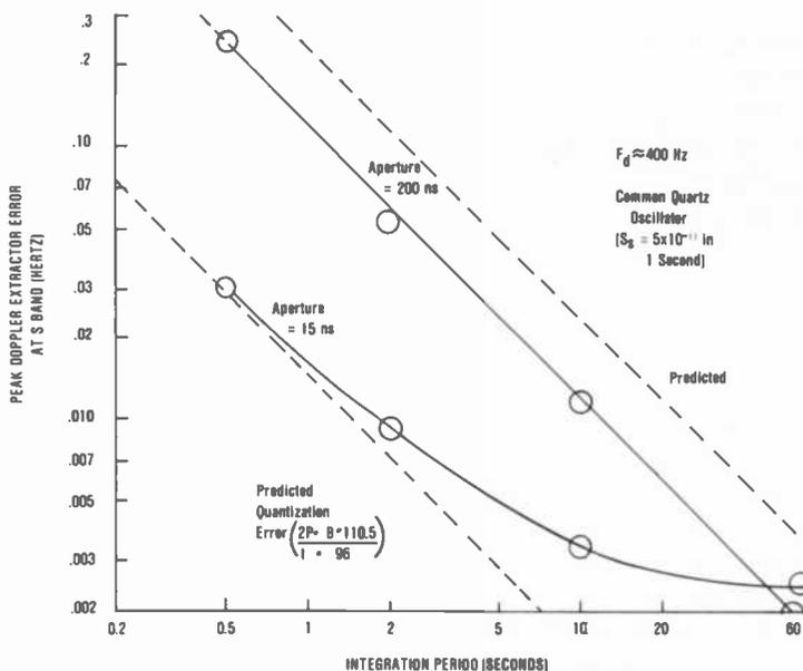
Fig. 18—One-way Doppler extractor measurement error.
