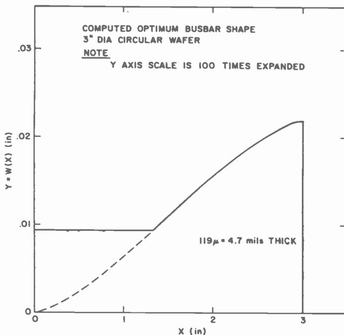
**Fig. 3—Computed optimum bus bar shape for a 3-inch diameter circular wafer. Area = 45.60 cm<sup>2</sup>, price of silver = \$1.30/cm<sup>3</sup>, array cost = \$0.0125/cm<sup>2</sup> (\$1/W). Note that the  $y$ -axis scale has been expanded 100 times.**
