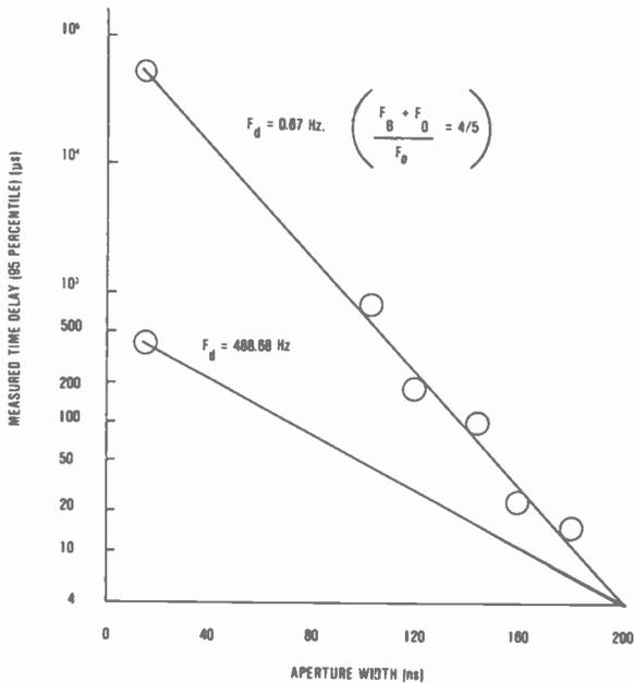
Fig. 20—Sensitivity of time delay to coincidence aperture and Doppler off-set.
