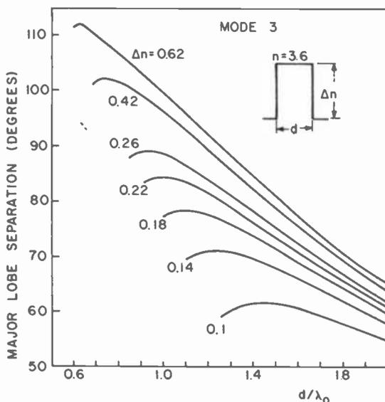
Fig. 6—Major lobe separation in the far-field for device operating in the third mode as a function of the index step  $\Delta n$  and  $d/\lambda_0$  (symmetric structure).
