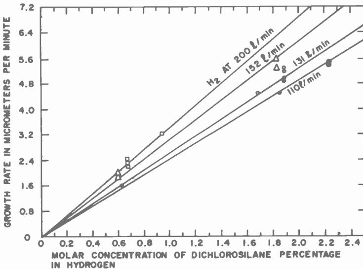
Fig. 1—Growth rate versus dichlorosilane concentration at various flow rates of hydrogen at 1050°C.
