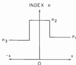
Fig. 2—Three layer dielectric model for the double-heterojunction laser.
