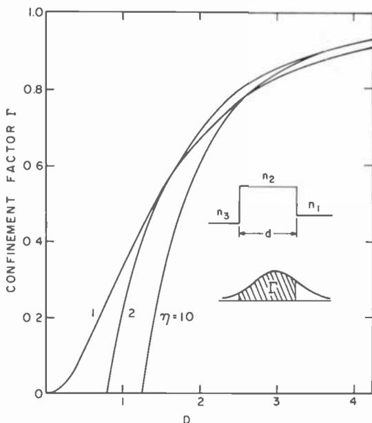
Fig. 12—The wave confinement factor  $\Gamma$  as a function of the normalized guide width  $D$  (see Eq. [7b]) for a symmetric DH laser ( $\eta = 1$ ) and asymmetry values  $\eta = 2$  and 10.
