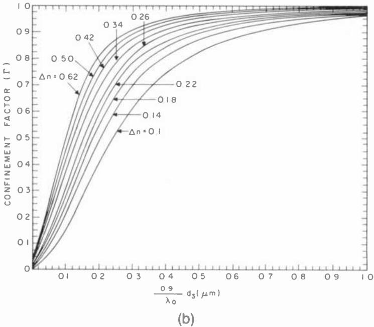
Fig. 11—Wave confinement factor  $\Gamma$  as a function of the effective guide width for (a)  $\Delta n = 0.04$  to 0.22 and (b)  $\Delta n = 0.10$  to 0.62.
