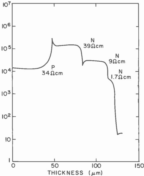
Fig. 3—Resistivity of epitaxial layers versus distance from substrate interface from spreading resistance measurements of a  $\pi$   $\nu$   $n$   $n^+$  structure.
