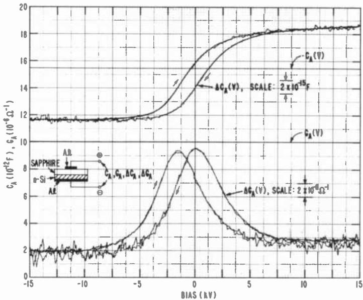
Fig. 10—Variation of capacitance and conductance with bias for an MIS sample fabricated from n-Si on sapphire.
