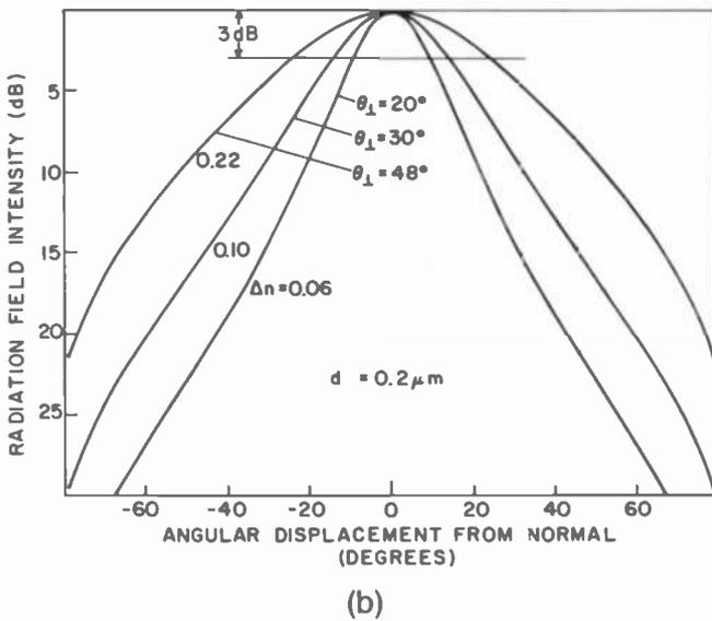
Fig. 8—(a) Field intensity as a function of  $\Delta n$  for  $d = 0.2 \mu\text{m}$ ; (b) corresponding far-field. Here  $\lambda_0 = 0.9 \mu\text{m}$ .
