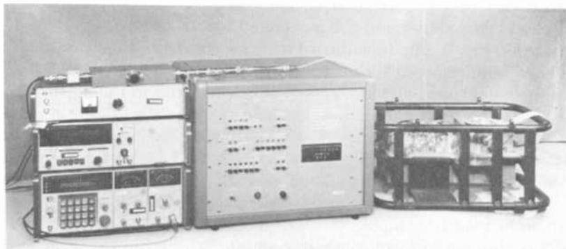
**Fig. 3—One-way Doppler extractor breadboard (center) and test instrumentation.**
