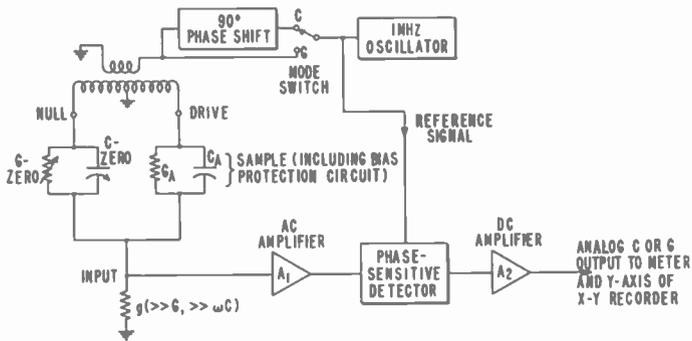
Fig. 3—Simplified equivalent circuit of C/G meter and BIU.
