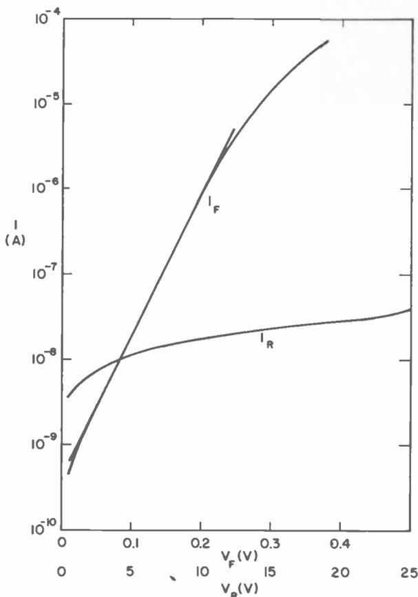
Fig. 2— $\log I_F$  versus  $V_F$  plot of a typical Al-SOS Schottky diode.
