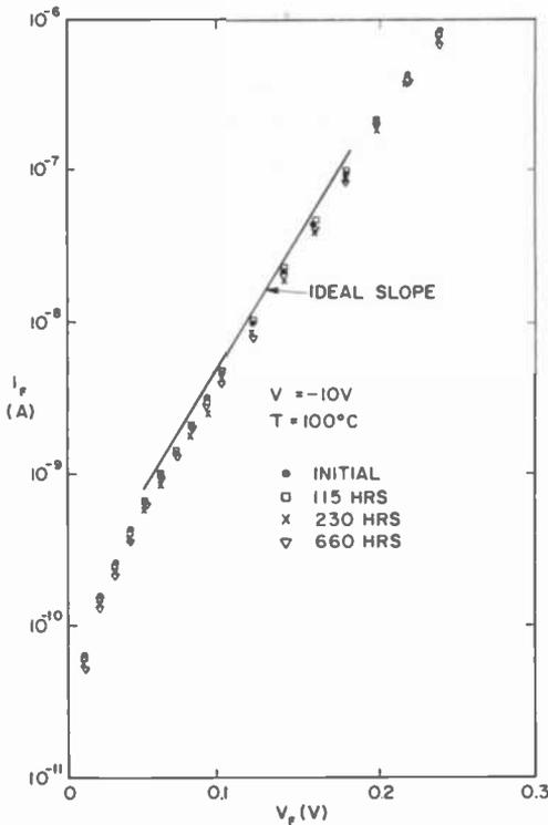
Fig. 4—The forward current-voltage characteristics of an Al-SOS Schottky diode before and after BT tests with  $V_R = -10\text{V}$ .
