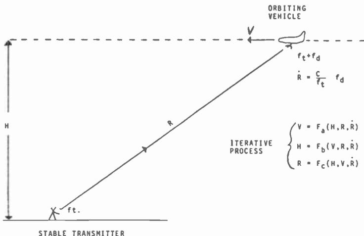
Fig. 1—One-way Doppler geometry.
