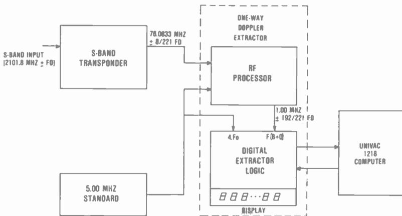
Fig. 14—One-way Doppler extractor interfaces.
