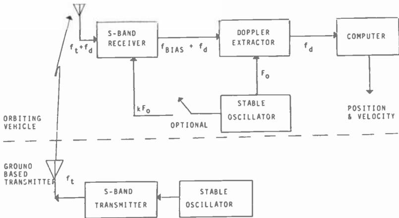
Fig. 2—Block diagram of a one-way Doppler navigation system.
