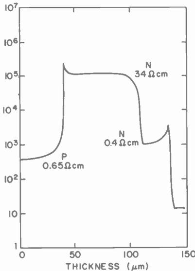
Fig. 2—Resistivity of epitaxial layers versus distance from substrate interface from spreading resistance measurements of a high voltage  $pn^{-}np^{+}$  structure.
