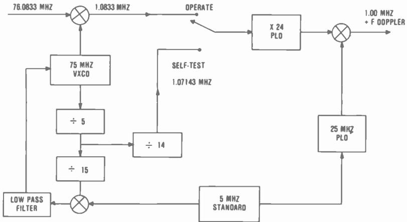
Fig. 16—Self-test implementation block diagram.
