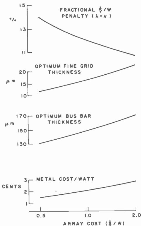
Fig. 2—Effect of total array cost in \$/W (plotted logarithmically) on several front metallization parameters of 3-inch diameter cells with screen-printed Ag lines having straight, parallel sides. The curve  $(\lambda + \kappa)$  is obtained from totals like those in Eq. [18].
