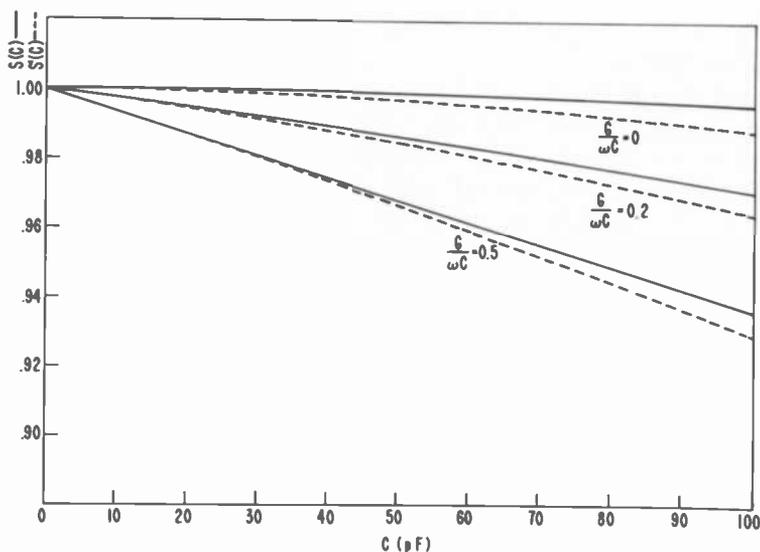
Fig. 5—Relative sensitivity factor  $S(C)$  and relative incremental sensitivity factor  $S'(C)$  versus  $C$ , with  $R = 100$  ohms and  $G/\omega C$  as a parameter.
