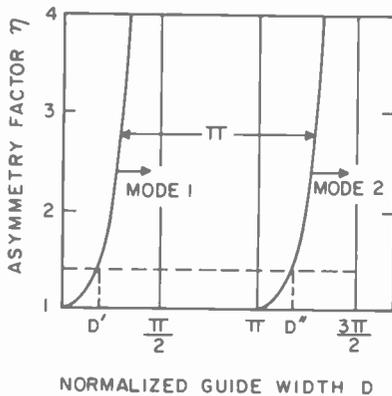
Fig. 3—Cutoff conditions for the first and second waveguide modes as a function of  $D$  (see Eq. [7b]). A waveguide geometry defined by a point to the right of each curve implies that the mode can propagate in the guide.
